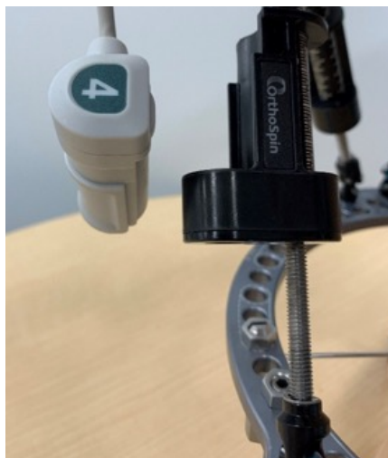
Figure 9: Picture of dislodged motor.
